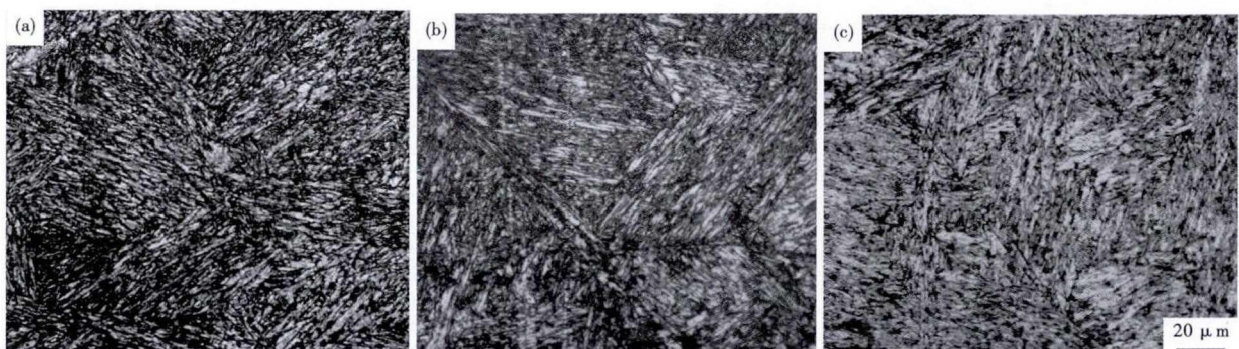
图 3 (a)950 °C,(b)1 040 °C 和(c)1 100 °C,淬火对 1Cr12Ni3Mo2VN 钢组织的影响,565 °C 3 h 回火 Fig. 3 Effect of quenching at 950 °C (a), 1 040 °C (b) and 1 100 °C (c) on structure of steel 1Cr12Ni3Mo2VN, tempered at 565 °C for 3 h
