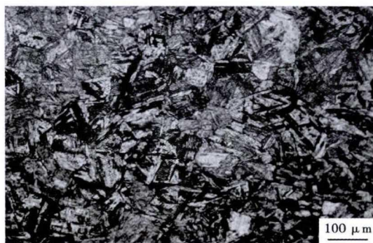
图 1 1Cr12Ni3Mo2VN 钢 \Phi 350 mm 锻材的组织形貌 Fig. 1 Morphology of structure of steel 1Cr12Ni3Mo2VN \Phi 350 mm forged product
